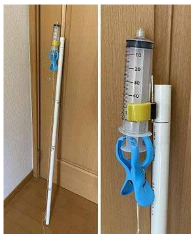
Fig. 2a: Water sampling rod
