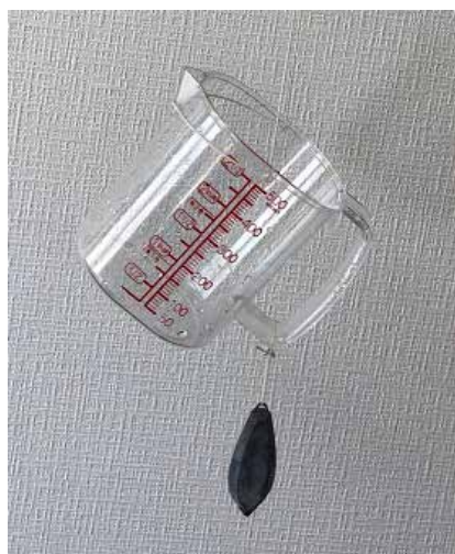
Fig. 1a: The modified cup for water sampling
