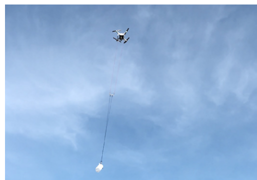
Fig. 3 Left: Drone water sampling. Right: enlarged image (Photo by Masayuki Sakata)
