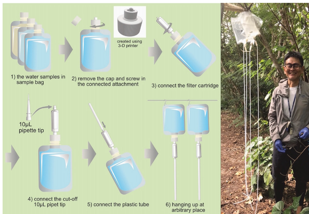
Fig. 1 Protocol set-up of the novel gravity filtration system for eDNA water samples. The photograph shows the filtration system hanging at about 2 m height in the field by Dr. Miya. [This figure is adopted from reference 2]
