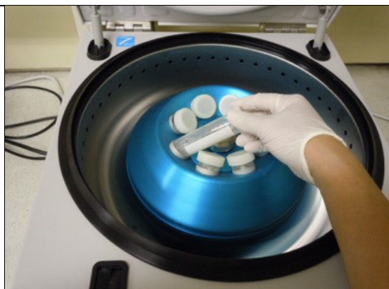
Fig. 4-1-3-9 Centrifuge the conical tube containing the Sterivex filter unit at 6000 g for 1 minute.
