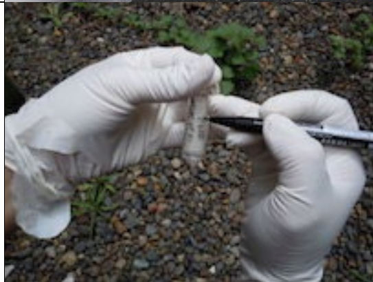
Fig. 3-1-2-15 Wipe the surface of the Sterivex filter unit with a paper towel, and write the necessary information, including sampling date and survey point number, on the Sterivex with a felt pen.
