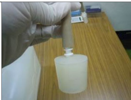
Fig. 3-1-3-4 Connect the rubber tube and the silicon with holes through the tube I joint (white joint).
